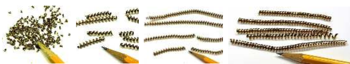
Fig 5: Representative chip forms collected during turning tests. ISO 3865 classifications from left to right are: CL 7 (elemental), CL 5.2 (short conical), CL 5.1 (long conical), CL 2.1 (long tubular).
